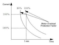
Fig.FA-1 Motor Overload Protection Factor
