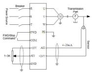
Fig. F8-1 Analog Feedback Control System
