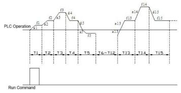
Fig.F9-2 Maintain Last Stage after Single Cycle
