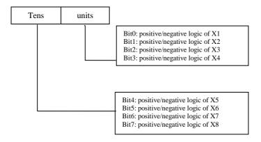
0: positive logic, which refers that the terminal Xi is enabled when it connects with the common port and disabled if disconnected.
