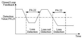
Fig. FA-4 Closed Loop Feedback Loss Detection
