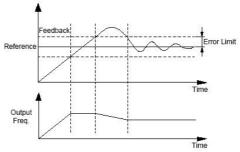
Fig. F8-3 Error Limit Schematic Diagram
