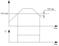
Fig.F7-8 Frequency Level Detecting
